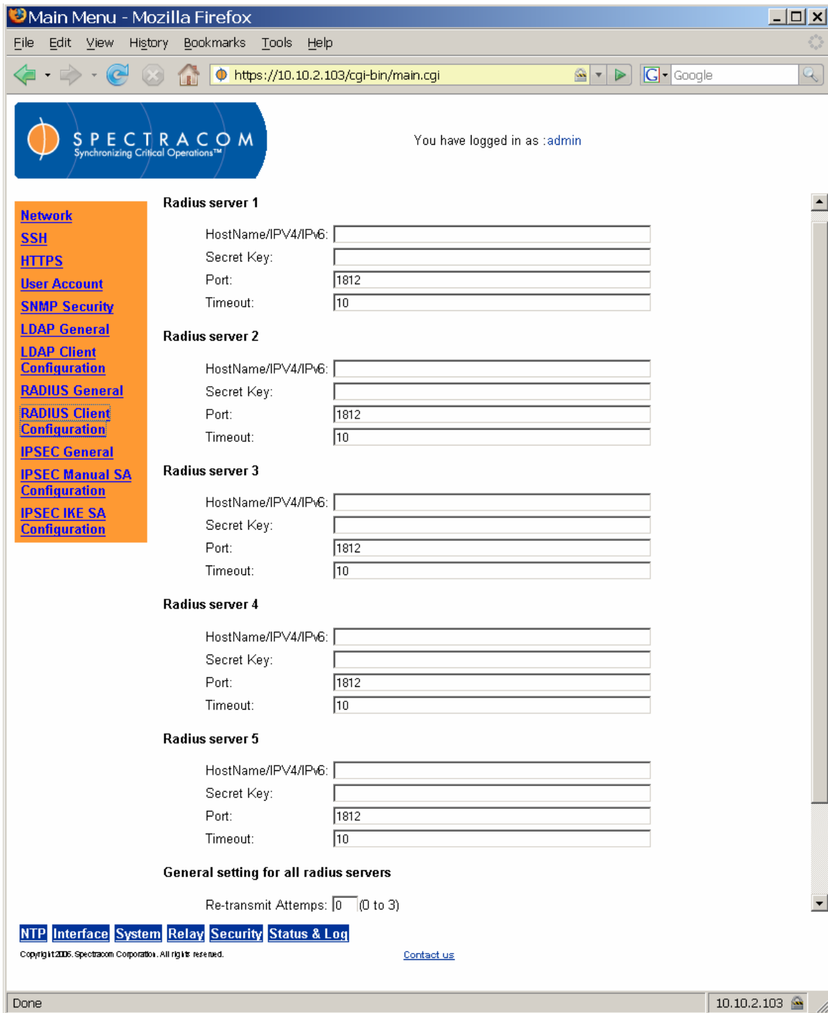
Figure 3-84: Security RADIUS Client Configuration Screen
