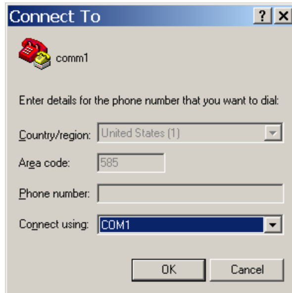
Figure 3-6: Connecting to the Computer's Serial Port
